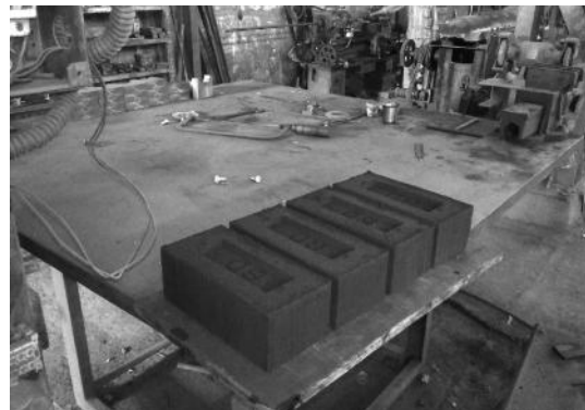
Trial run for manufacturing of bricks containing CETP Sludge
